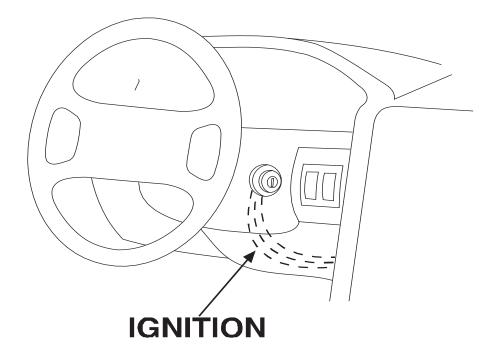
Once the lower dash panel has been removed, locate the ignition harness at the back of the key cylinder. This is usually a group of heavy gauge wires (approximate 14ga.).
